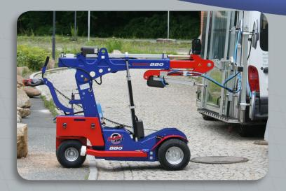
When your project requires a slightly larger unit, the MAVLift 880 is ready for service. Offering the MAVLift's signature Synchronous Controls that keep the suction unit at a constant inclination angle automatically, the MAVLift 880 preforms with precision while lifting up to 880 lbs on a compact chassis measuring less than 3 feet across.
