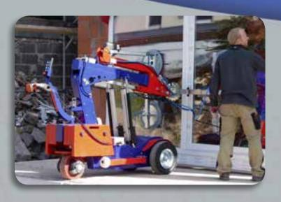
When your project requires a slightly larger unit, the MAVLift 880 is ready for service. Offering the MAVLift's signature Synchronous Controls that keep the suction unit at a constant inclination angle automatically, the MAVLift 880 preforms with precision while lifting up to 880 lbs on a compact chassis measuring less than 3 feet across.
