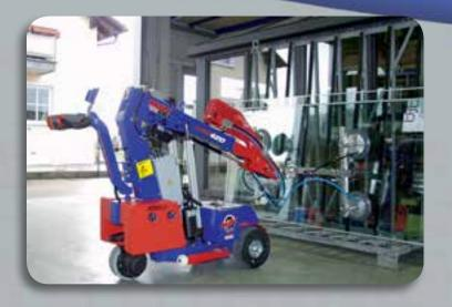
The smallest of the traditional Indoor Glass Robots, the Indoor 620 is the perfect glazing tool for installing glass or moving materials weighing up to 620 pounds.
